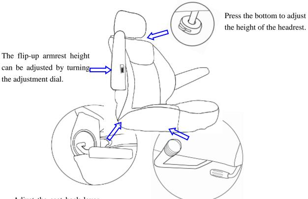
Adjust the seat back lever for seating back angle.
